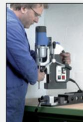
Using the portable clamping mechanism, MobilCLAMP, you can supplement the application options of a magnetic core drilling machine onsite and in the workshop. The magnetic core drilling machine is placed on the desired surface for this purpose
