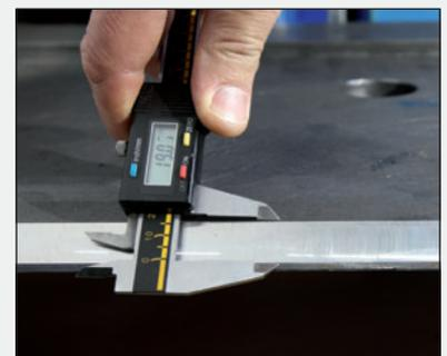
Chamfer width 30 mm max.
