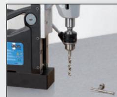
Twist drills up to ø 18 mm
