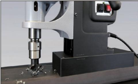
**Countersinking from  $\varnothing$  80 mm – reaming to  $\varnothing$  50 mm.** BDS magnetic core drilling machines with MT tool holder are adapted for the universal use of reamers and countersinks. An overview can be found on pages 10 and 11.
