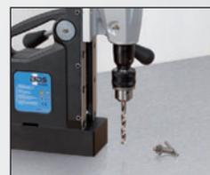
Twist drills up to ø 13 mm
