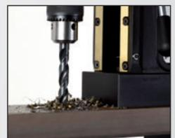
Twist drilling up to  $\varnothing$  31.75 mm
